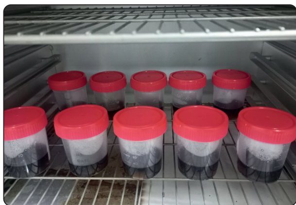
Fig. 4: Samples immersed in coffee solution inside incubator
