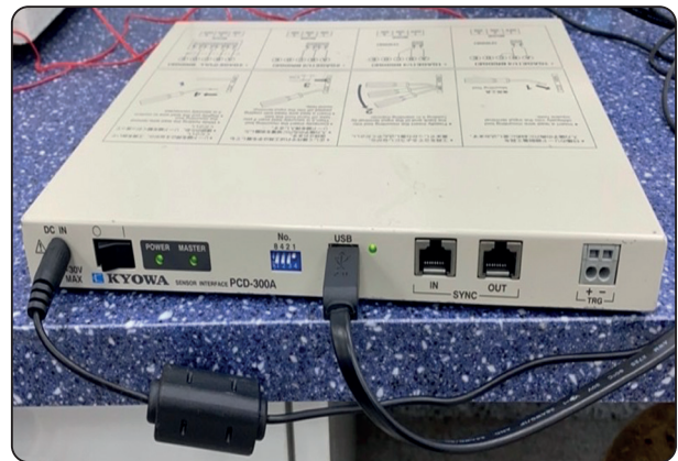
Fig. (6) Four channels strain meter.
