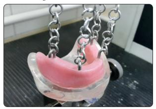
Fig. (4) Four hooks are connected to chains for measurement of retention.
