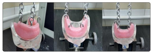
Fig. (5): Application of displacement forces, lateral, posterior and anterior respectively.
