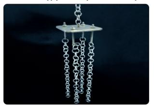
Fig. (3) Four chains and metal plate that was connected to the testing machine to apply different displacement forces.
