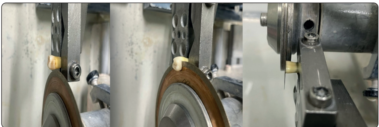
Fig. (1): Coronal Sectioning using IsoMet
