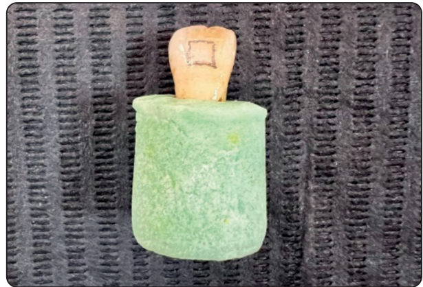
Fig. (1) The roots of the teeth were placed in molds of acrylic resin
