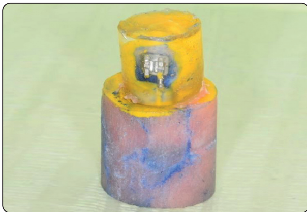
Fig. (2) A sample ready for sectioning for microleakage evaluation
