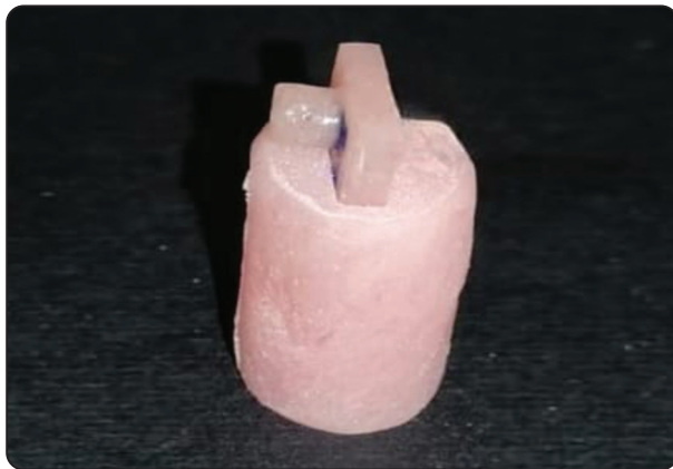
Fig. (3) To facilitate attachment to the Universal testing machine, all specimens were attached to a cylindrical self-cured acrylic resin holder of dimensions 1.8cm length and 1.5cm diameter.
