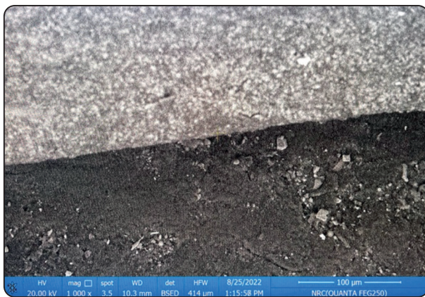
Fig. (2) SEM image at 1000X showing the complete adaptation of En70 crown margins on the typodont tooth.
