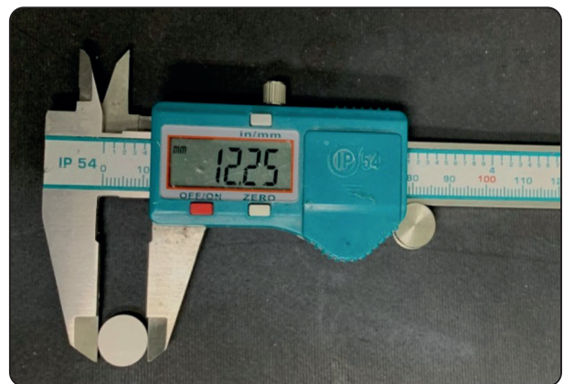
Fig. (2) Disc diameter checking before sintering
