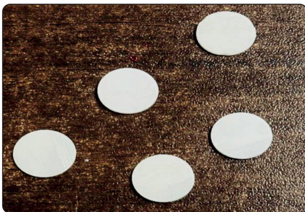
Fig. (1) Discs after ISOMET cutting
