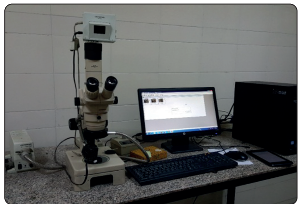
Fig. (6) CCD digital camera mounted on stereomicroscope.
