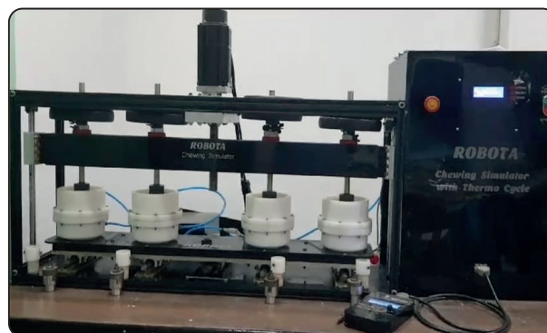
Fig. (2) Four stations multimodal ROBOTA chewing simulator
