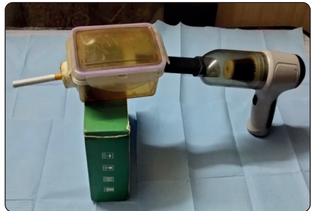
Fig (1) A custom-made chamber device consisted of a vacuum system directing the smoke to the specimen inside a plastic box
