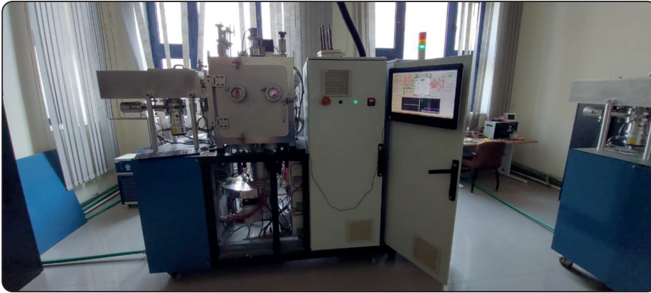
Fig. (1) PROTOFLEX physical vapor deposition platform, Faculty of Nanotechnology for postgraduate studies, Cairo University, Cairo, Egypt., used for coating mini screws with zinc oxide NPs.
