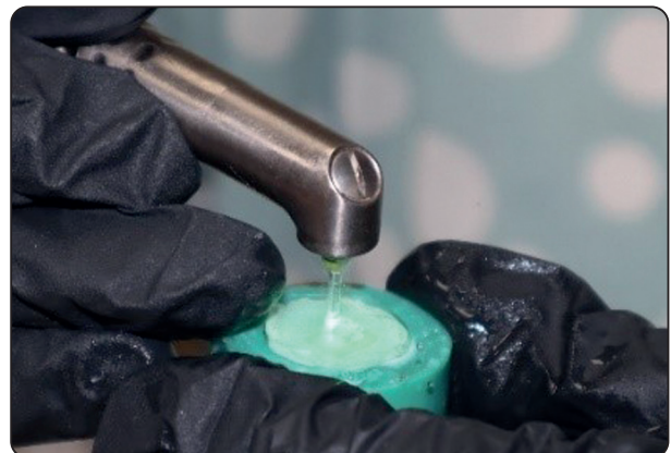
Fig. (2) Ceramic bracket lased with Er,YAG laser
