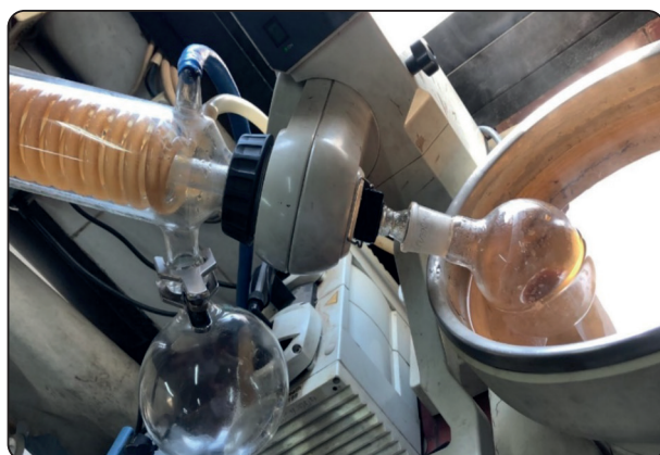
Fig. (2) The extract concentration procedure using Rotavapor
