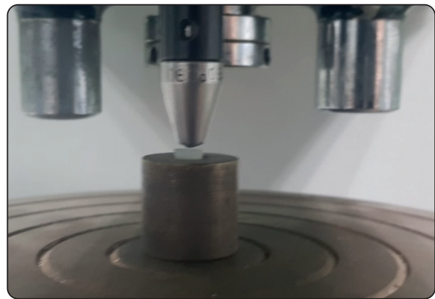
Fig. (2) Vicker hardness test for measuring microhardness
