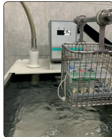
Fig. (2) A thermal cycling simulation device
