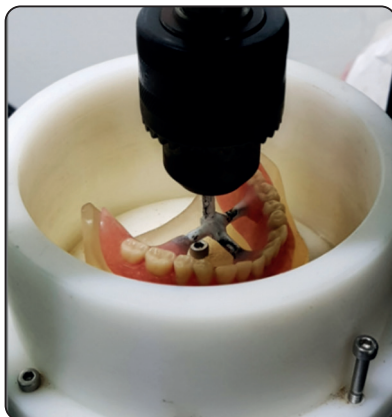
Fig. (19) Denture in place on the chewing simulator
