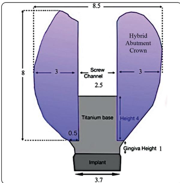
Fig. (1) Schematic diagram for the dimensions of the hybrid abutment crown
