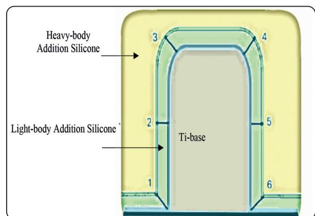
Fig. (4) Diagram representing points of internal fit measurements
