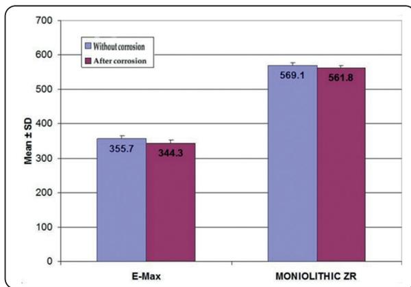
Fig. (3) Comparison between the micro hardness of tested ceramics
