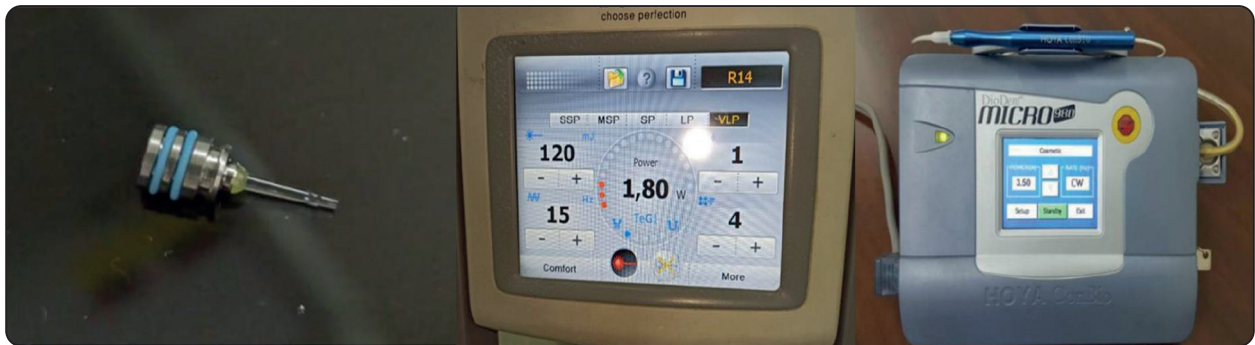
Fig. (1) Components and parameters of the laser systems used in this study. (A) Fiber tip of the Er: YAG laser with specifications: sapphire, conical 8/0.8, Fotona® part number 72560, fiber tip efficiency 100%, maximum laser energy 350 mJ. (B) Operational settings and laser parameters of the Er: YAG laser system. (C) Operational settings and laser parameters of the Diode laser system.
