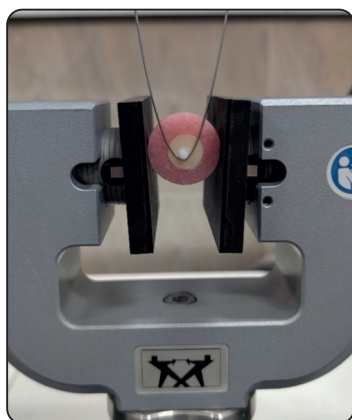
Fig. (2) Micro shear bond testing using Universal testing machine.
