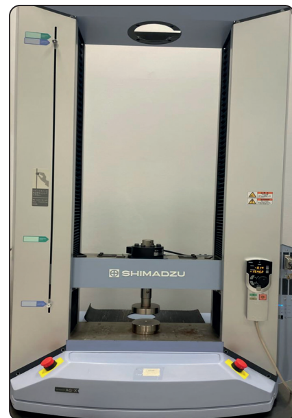
Fig. (4) Universal testing machine with the specimen aligned horizontally
