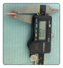
Fig. (4): Caliber checking 2 mm thickness of slices samples
