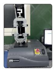
Fig. (1): Instron machine used in push out test
