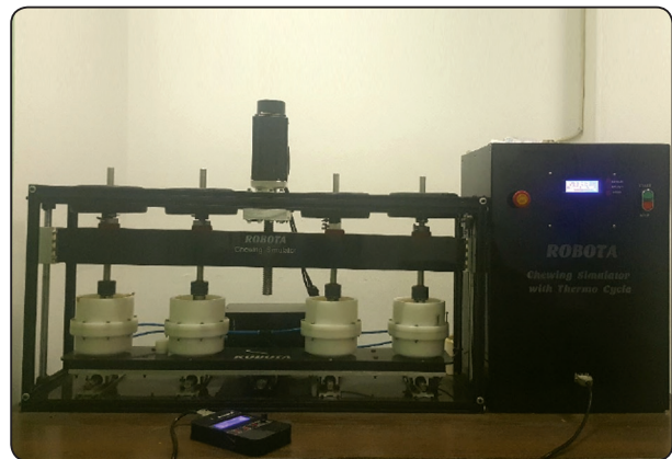
Fig. (2) Robota chewing simulator for thermomechanical aging
