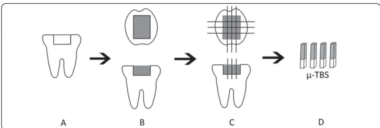
Figure 1: Schematic illustration of specimen preparation in high C-factor cavity.
