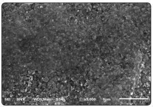
Fig. (5) SEM micrograph (5000x) showing the zirconia surface after etching with hot acid solution and Silano-Pen treatment.
