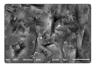
Fig. (2) SEM micrograph (5000x) showing the air abraded surface of zirconia.
