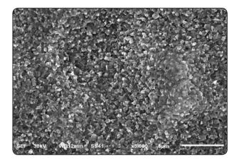
Fig. (4) SEM micrograph (5000x) showing the zirconia surface after etching with hot acid solution.
