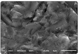
Fig. (3) SEM micrograph (5000x) showing the zirconia surface after etching with Piranha acid solution.
