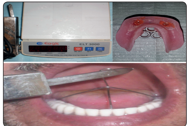
Fig. (4) Digital Forcemeter & snap hooks attached to geometrical center of denture for retention measurement
