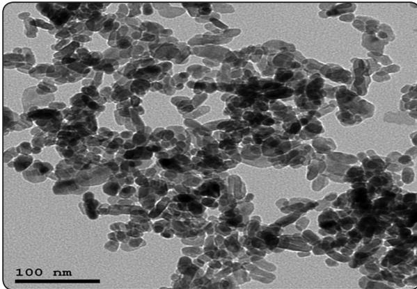
Fig. (1): TEM image represent the morphology of zinc oxide Nanoparticles
