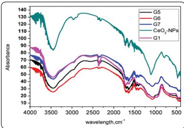
Fig. (5): FTIR spectra of the CeO2-NPs, GI and GI incorporated with different concentrations of CeO2-NPs
