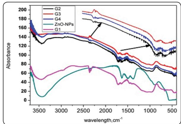
Fig. (4): FTIR spectra of the ZnO-NPs, GI and GI incorporated with different concentrations of ZnO-NPs
