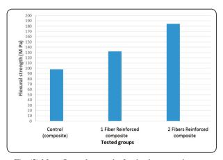
Fig. (2) Mean flexural strengths for the three tested groups
