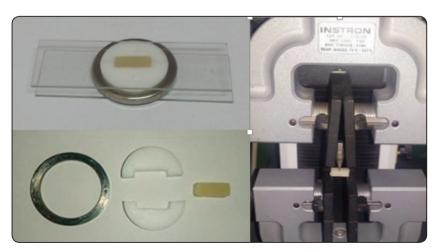
Fig. (1) Preparation and testing of the specimens.
