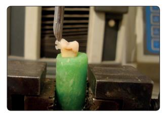
rod attached to the upper movable compartment of testing machine. The chisel tip positioned to touch only the base of the bracket. The maximum failure load was recorded in N.
