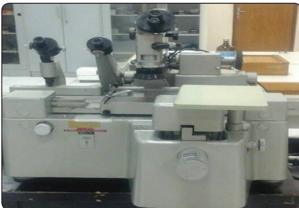
Fig. (5) The travelling microscope used for gap measurements
