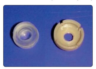
Figure (2): Right: Nylon Matrix, Left: PEEK Matrix with hole and slits
