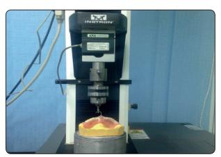
Fig. (3): Denture in place with attached wires forming a loop at the geometrical center and attached to the universal testing machine.
