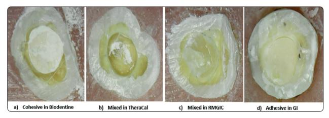
Fig. (4) Representative stereomicroscopic images for different failure modes within all groups (× 25)
