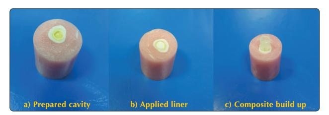
Fig. (1) Steps of shear bond strength sample preparation
