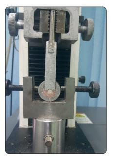
Fig. (2) Shear bond strength sample mounted onto testing machine
