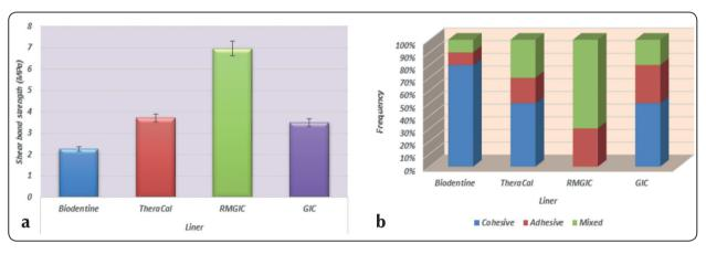
Fig. (3) Shear bond strength means values (3:a) and failure mode distribution (3:b) for liner groups
