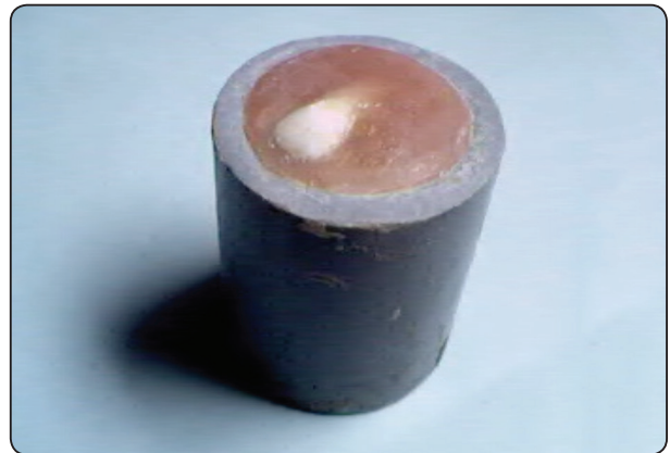
Fig. (1) Tooth invested into metal ring using self-curing acrylic resin.
