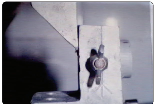
Fig. (2) Shear dislodging force applied via a knife edged metal bar attached to the upper member of the testing machine.
