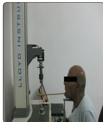
Fig. (2) Measuring retention using universal testing machine
