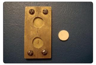
Fig. (1) Split circular brass mold used to create disc samples.
