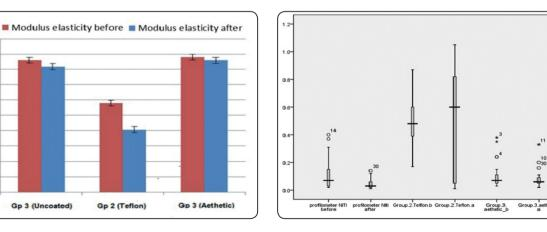
Fig. (3): Error bar chart for Modulus of Elasticity of the studied wire groups
