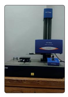
Fig. (2): The surface profilometry
