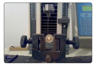
Fig. (5) One end of the wire is attached to the machine and the other path through the bracket
