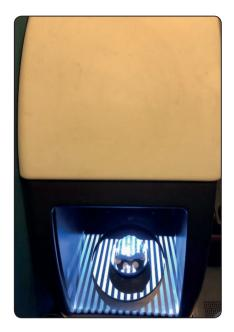
Fig. (2) Optical Scanner – Open Technologies while scanning a dental model
