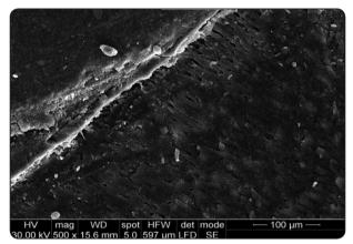
Fig. (3e) ESEM photomicrograph (500X) for Immediate dentin sealing with removal of O2 inhibited layer and finishing before cementation (IDS2) showing intact interface with a relatively thin cement line and hybrid layer
