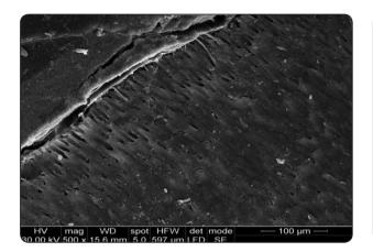
Fig. (3i) ESEM photomicrograph (500X) for Immediate dentin sealing without removal of O2 inhibited layer and with finishing before cementation (IDS4) showing intact interface with evidence of few resin tags
