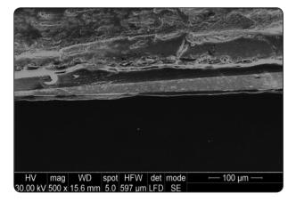
Fig. (3a) ESEM photomicrograph (500X) for Delayed dentin sealing (DDS) showing absence of gap formation and variable cement line thickness
