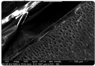
Fig. (3h) ESEM photomicrograph (500X) for IDS3 group after thermocycling showing showing presence of definite gap between the relatively thick hybrid layer and the cement.
