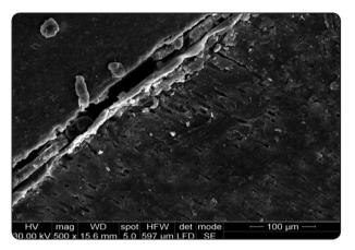
Fig. (3f) ESEM photomicrograph (500X) for IDS2 group after thermocycling showing presence of gap in some parts of the interface with evidence of few long and very thin resin tags.
