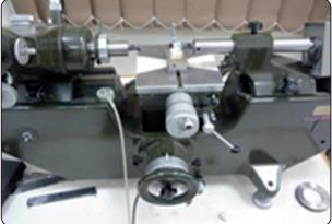
Fig (2): Universal horizontal metroscope
