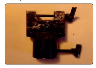
Fig (5) Showing Two custom made metallic hooks were fabricated to be fixed to the upper and lower parts of the Instron machiene.
