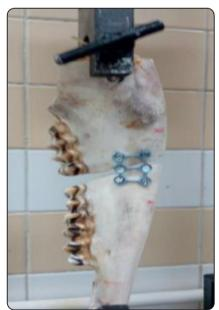
Fig (6) ShowingThe custom made tension test device was attached to the testing machiene and was used for compression test for Group (2) prepared samples.
