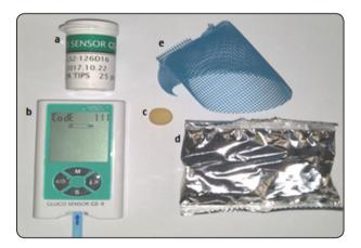
Fig. (3) Gluco Sensor Set. a, sensor tips package; b, measuring set; c, chewing specimen; d, chewing specimen package; e, plastic filter
