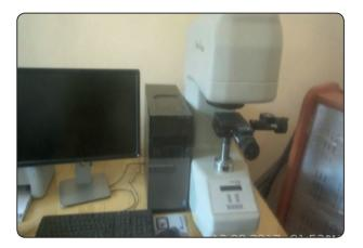
Fig. (1) Indentation hardness tester (Zwick. roell, system 5153. UK).
