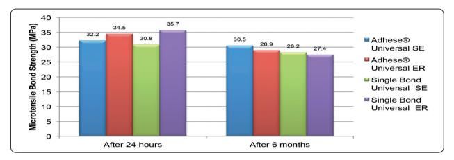
Fig (1): Column chart showing the mean dentin µ-TBS (MPa) for different adhesives and bonding approaches within each aging time
