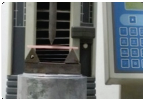
Fig. (1) Flexure strength test sample loaded onto universal test machine.
