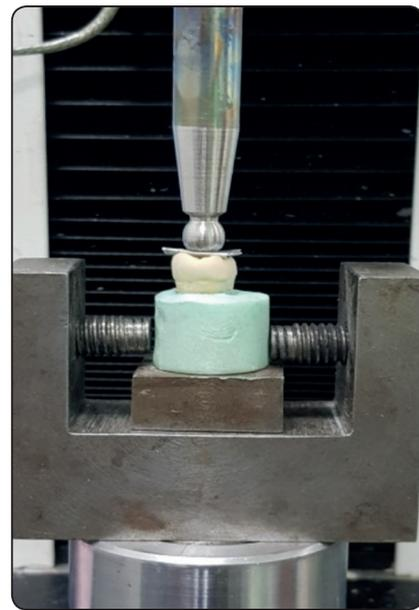
Fig. (4): Universal testing machine applying load on to the endocrown
