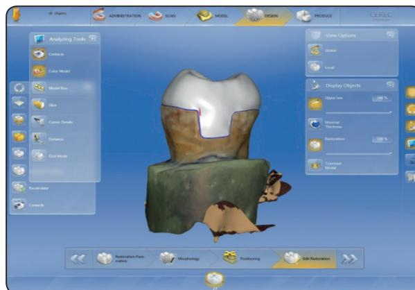
Fig. (3): on screen image of the final designed endocrown restoration
