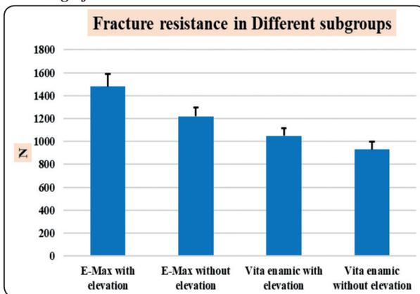
Fig. (6): Bar chart of mean fracture resistance in different subgroups
