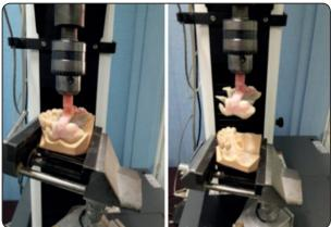
Fig. (4) insertion-removal test
