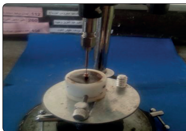
Fig. (1) The dowel aligned perpendicular to the base of the acrylic mold by dental surveyor
