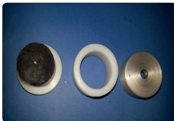
Fig (2) A black acrylic cylinder with the fiber post in Teflon rings and a metal device
